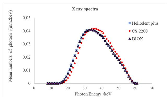
**Figure 4** Spectra of DIOX - Portable Radiographic Dentistry Device compared to conventional CS 2200 and Heliodent plus- Sirona.
