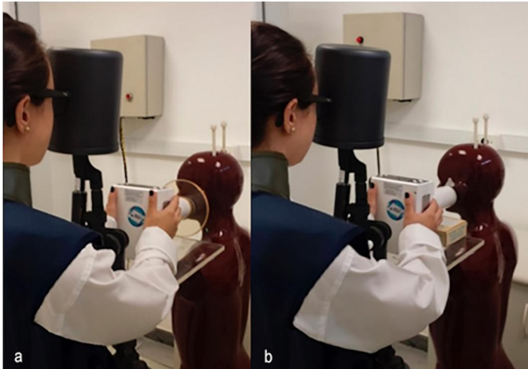
**Figure 1** Simulation of the upper left molar periapical examination using the RANDO Alderson simulator: (a) With acrylic protector (b) without acrylic protector
