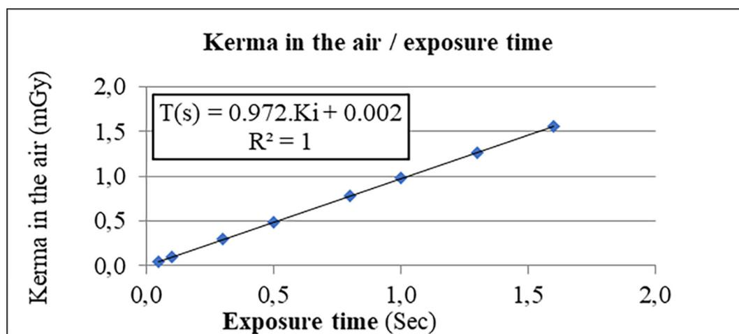
**Figure 3** Kerma in the air Linearity as a function of exposure time.
